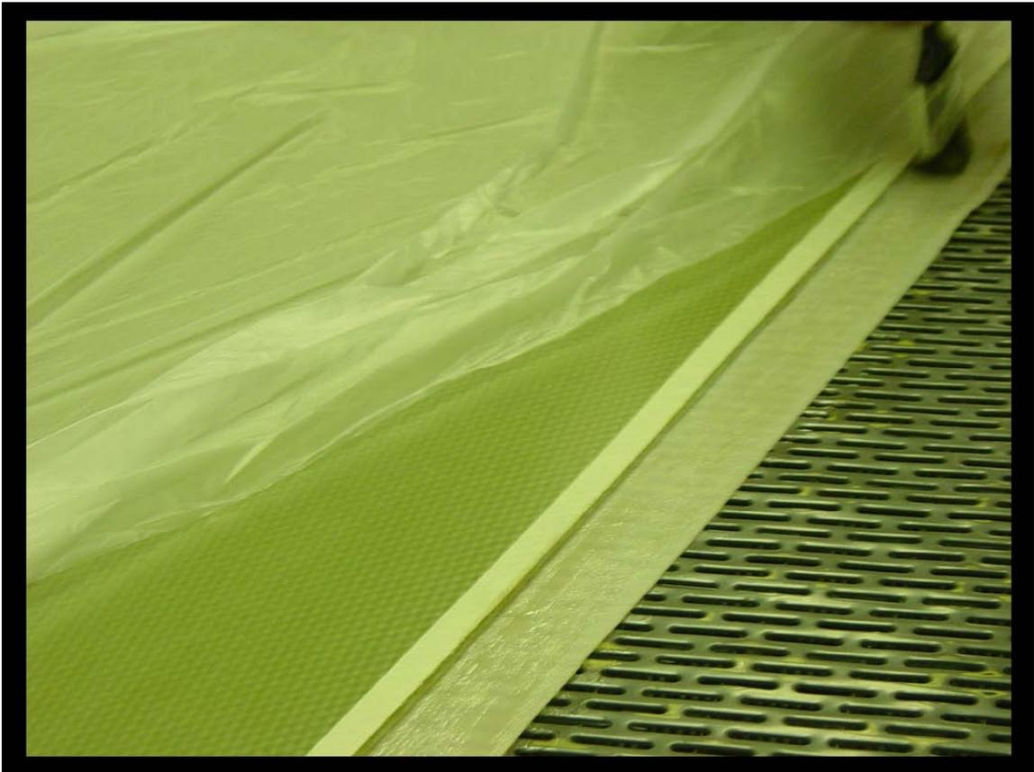
8. Lay plastic film over the freshly glued lower flap. The glue is industrial grade contact cement and will bond the belt together instantaneously. The plastic film allows the two flaps of the freshly glued joint to be aligned before the joint is bonded together.
